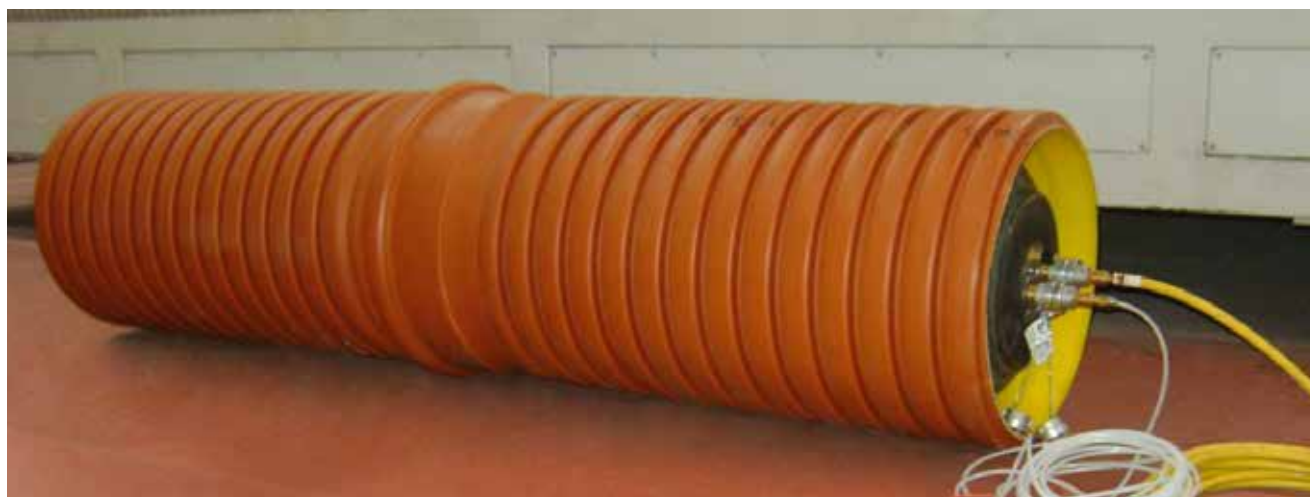
Coupling seal test according to UNI EN 1277: the test verifies the Kingcor pipe coupling system performance under critical situations in which the socket may be deformed.
