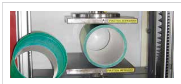
Test for annular rigidity determination on a sample of ecopozzo
